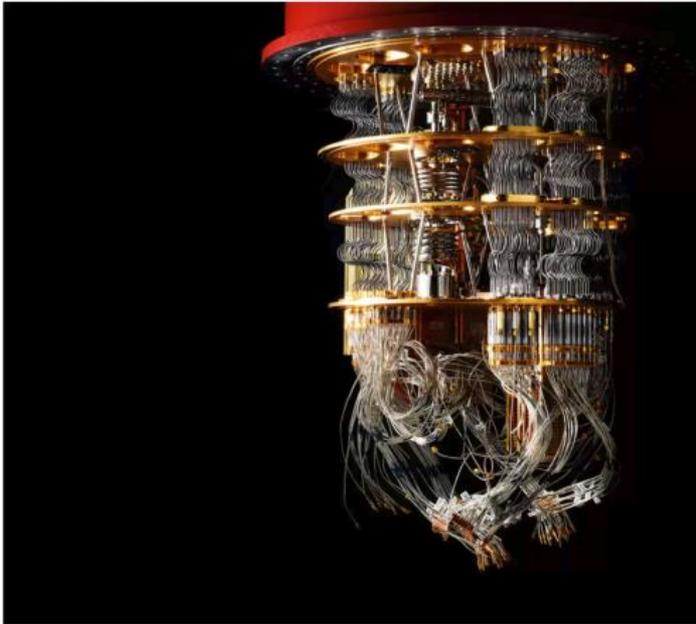
A cryostat at Google's quantum computing lab near Santa Barbara, California designed to keep a quantum chip at 10 millikelvin.
